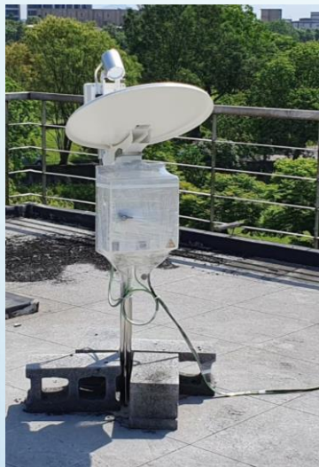
Microwave Rainfall Radar
