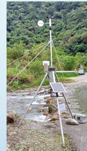
Mobile Automatic Weather Station
